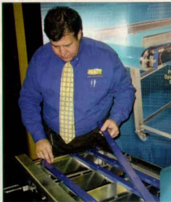
Plastic guides for the belt lift out without tools in MSE's sanitary conveyor frame. Source: MSE.
